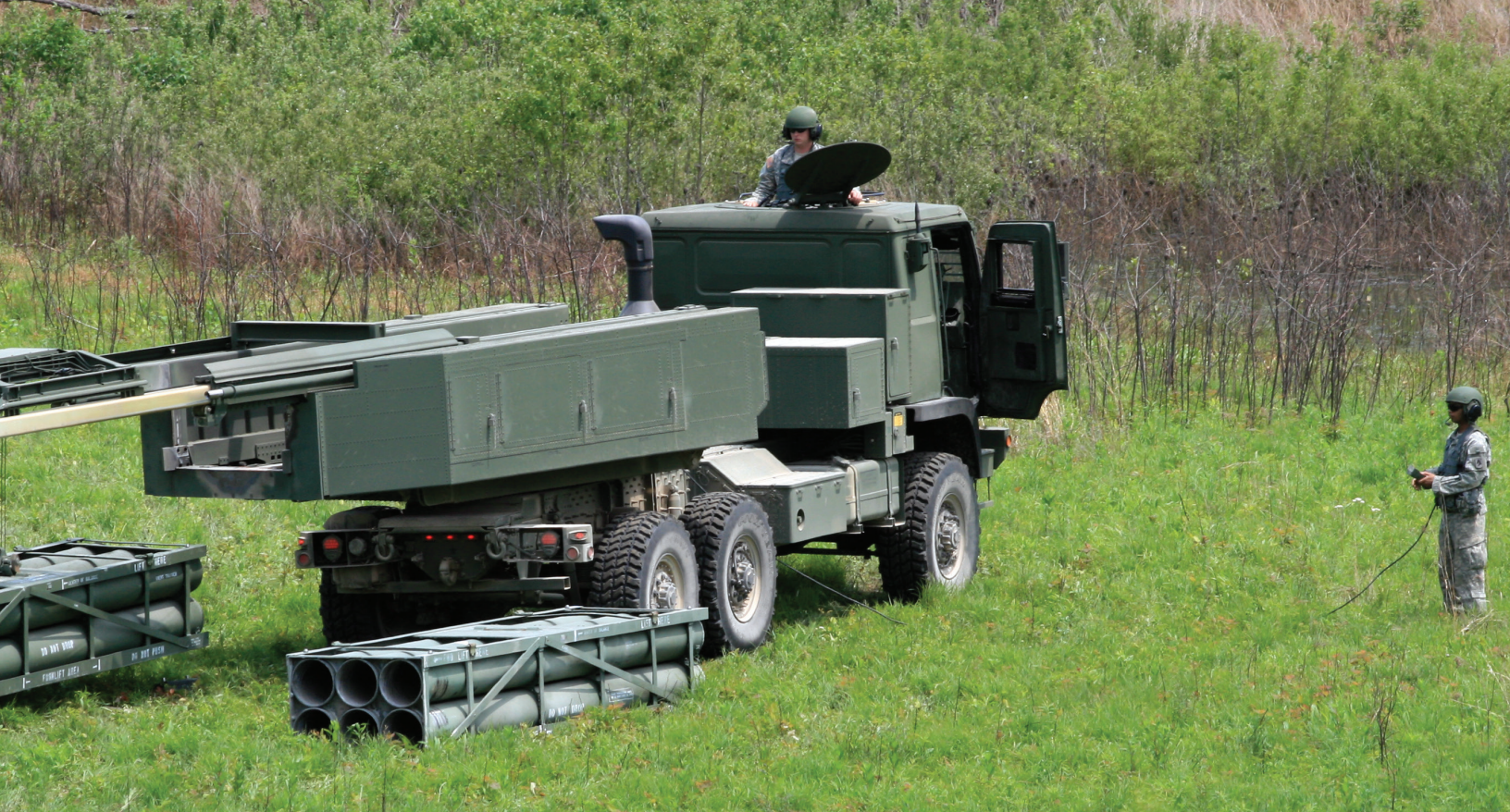
A HIMARs firing crew loads live pods at an ammunition reload point during the live-fire exercise May 15 at Fort Knox. Each weapon system can hold six rockets with an effective firing range of 120-186 miles.
